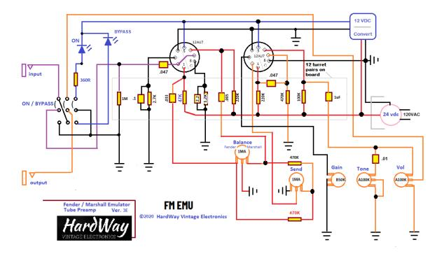
The layout of the FM EMU chassis is straightforward, and incorporates a true bypass switch, power indicating LEDs, and a 24V to 12V converter.
