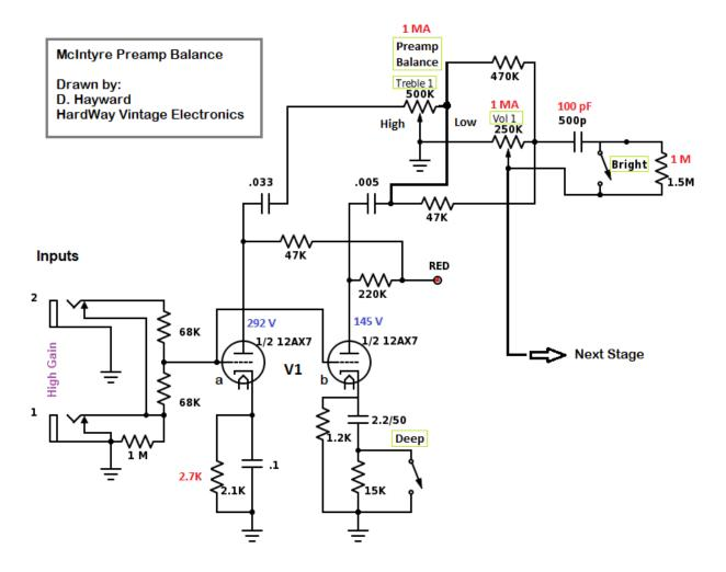
In the McIntyre design, triode V1a is very "Fender-like", while V1b is very "Marshall-like". The guitar signal's parallel input is subsequently blended between the two gain stages before heading for the next gain stage.
