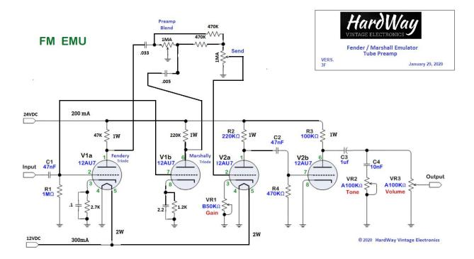
In the HardWay FM EMU design, there are dual power supplies – 12VDC for the tube filaments and 24VDC for the B+ voltage.
